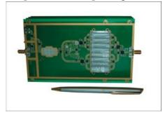
RS/DC 3-19 converter is designed as a heterodyne receiver with a preselector. 3.0...19 GHz frequency range is covered by 8 input filters with 2.0-2.5 GHz bandwidth.
