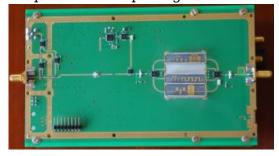
RS/DC 3-12 converter is designed as a heterodyne receiver with a preselector. 3.0...12 GHz frequency range is covered by 4 input filters with 2.0-2.5 GHz bandwidth.
