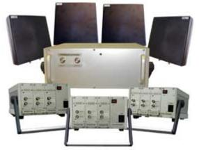
This system is more accessible for private buildings with a lot of little rooms, cabinets and etc. and where it is necessary to eliminate all using mobile phones.
